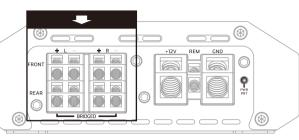
insert them into the block terminal while being careful that there is no loose or frayed strands of wire and tighten the Allen head screw down on the terminal till the wire is tightly secured in place.If the wires ever come in contact with each other the amplifier will go into protection.
